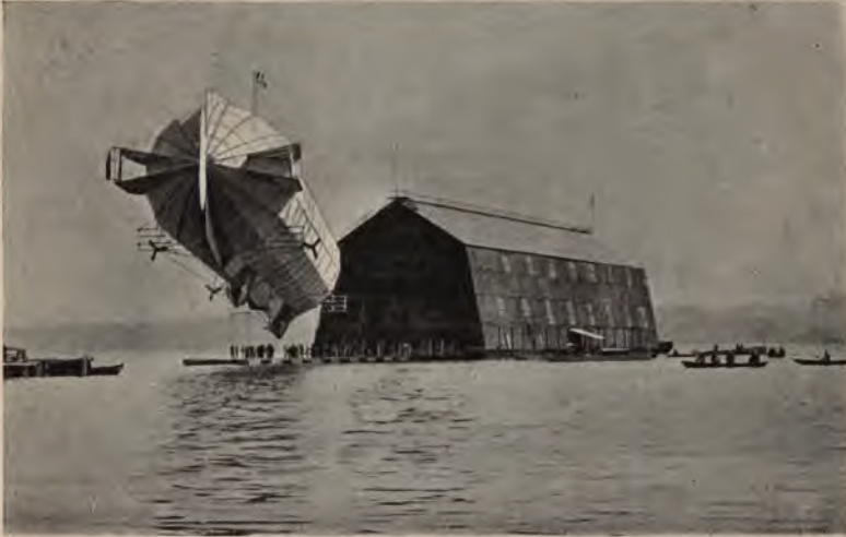
Fig. 92.—Count Zeppelin's aluminium-covered airship coming out of its shed on Lake Constance.
